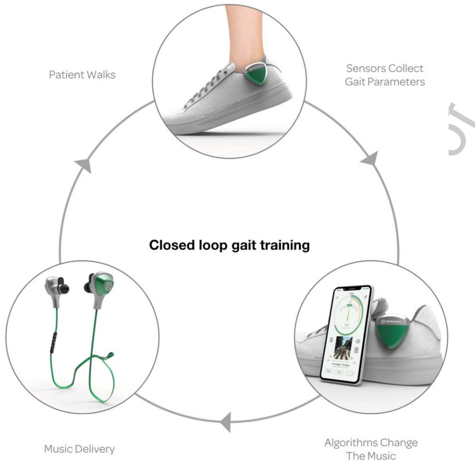
Fig. 1. Digital Closed Loop Gait Training Therapeutic In the top portion of the figure, a sensor is worn on the shoe to collect real-time walking cadence. A smartphone (lower right) houses the music playlist and delivers the acoustic signals through headphones worn (lower left) by the patient. Algorithms time shift the music to match the patient's cadence and modulate according to entrainment outcomes.
