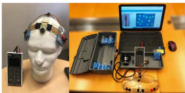
Figure 1: Tele-monitored tDCS (tele-tDCS) setup including the tDCS device, head strap and the videoconferencing platform.
