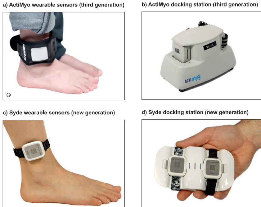
Fig. 1. Wearable magneto-inertial sensors: The third-generation ActiMyo (a and b) is succeeded by the new-generation device (Syde; c and d) which will be used in patients from 2021. Ambulant patients can wear a sensor strapped to each ankle, or one on the wrist and one on the ankle; sensors capture data throughout the day. The devices are transferred to a docking station overnight and the encrypted, anonymized data can be sent via a secure web cloud or stored on the internal USB drive [13]. The new-generation device (c and d) was redesigned with input from patients and healthcare professionals; it maintains the same level of sensor performance and measurement precision as its predecessor (a and b) but is one-third of the size and half the weight. The data recording station has also been modified to enable data capture for up to two weeks without internet connection or battery charging. Image a ©PhotoRoom.
