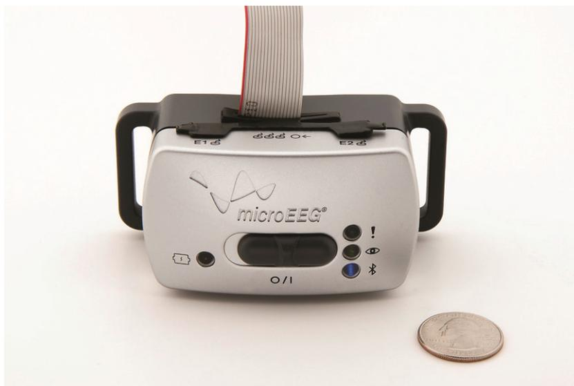
Fig. 1. The *microEEG* EEG device.
