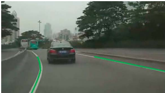
Fig. 6. Fitting the lane lines.
