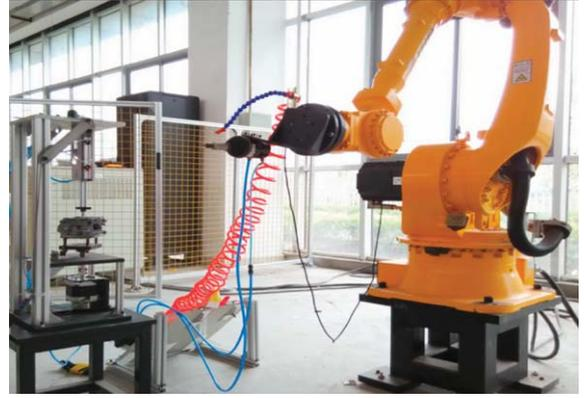
Fig. 1. The deburring industrial robot system.
