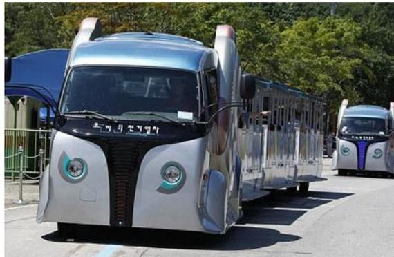
**Fig. 2. OLEV Tram installed in Seoul Grand Park.**
