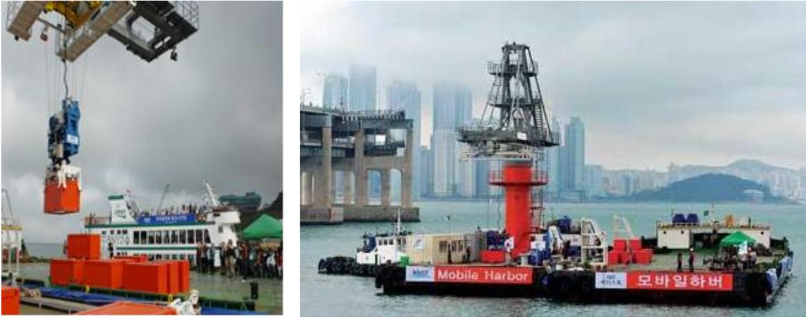
Fig. 3. 1/3 scale mobile harbor A1-250 developed at KAIST.
