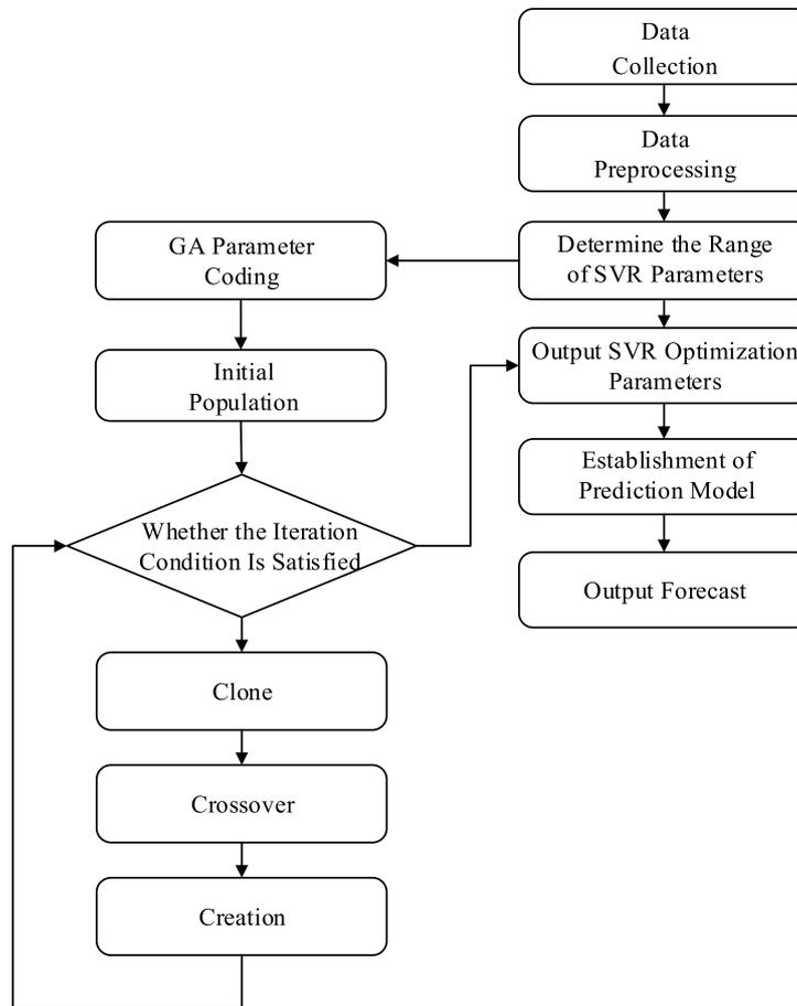
Fig. 1. GA-SVR traffic flow forecasting method flow chart.
