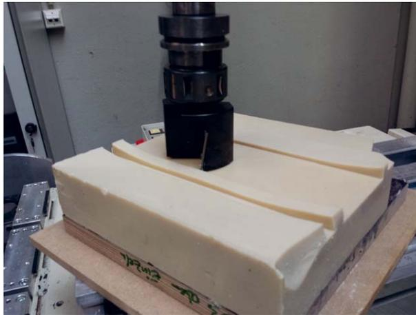
**Fig. 6.** Processing of technical wax by milling. (C) Sarah Baron, IWF Institute of Machine Tools and Manufacturing, TU Braunschweig.
