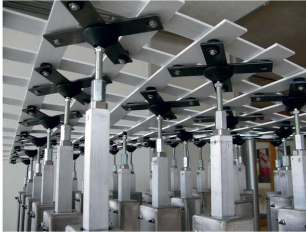
**Fig. 5.** First prototype of an adjustable mould.
