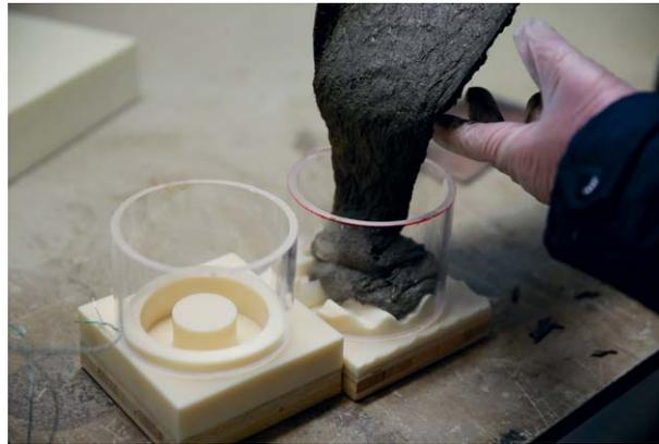
**Fig. 7.** Principle of wax formwork technology - Wax moulds are filled with UHPFRC (C) by Jeldrik Mainka, Institute for Structural Design (ITE), TU Braunschweig.
