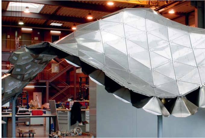
**Fig. 4.** Example of incremental sheet forming (C) by David Bailey Institute of Metal Forming IBF, RWTH Aachen University, Germany.
