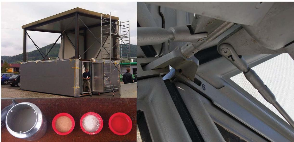
**Fig. 24.** Sand, dust, and seawater was brought from Abu Dhabi and sprayed on full-scale components during life cycle tests. Inside a controlled testing chamber the dynamic unit was monitored over 30,000 cycles. This was the equivalent of eighty years of operation compressed into two months.
