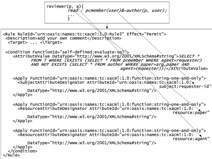
Fig. 17. A formula in a RW script and its generated conditions.
