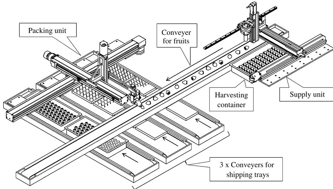
Fig. 3. Schematic diagram of automatic packing robot for strawberries [23].
