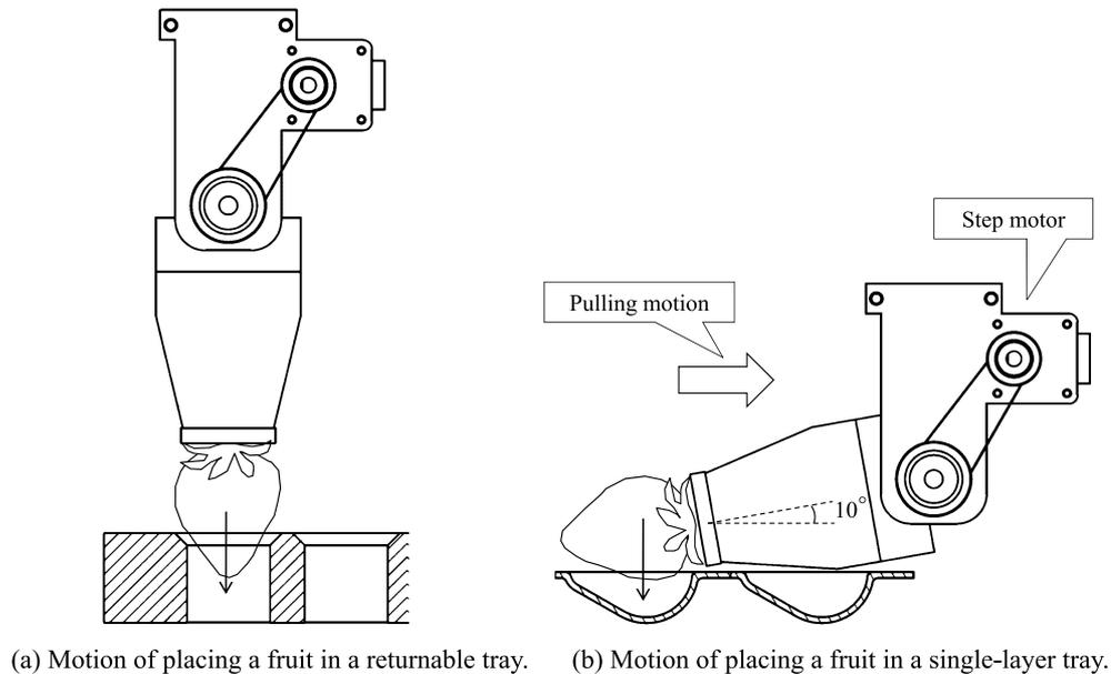
Fig. 4. Tilt motion of the packing unit's suction device [23].
