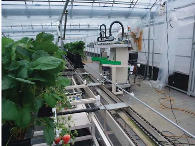
Fig. 7. Stationary-type strawberry-harvesting robot.
