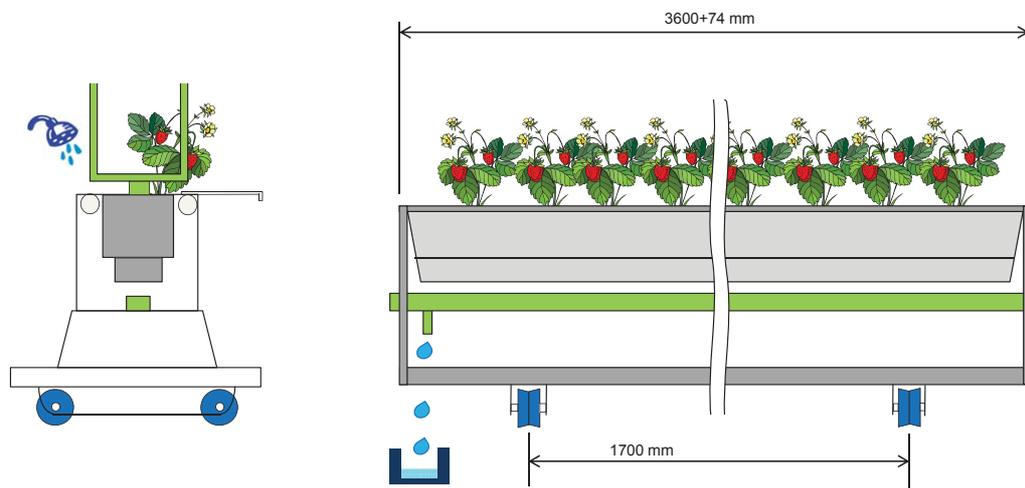
Fig. 6. Schematic diameter of planting bench for movable bench system.
