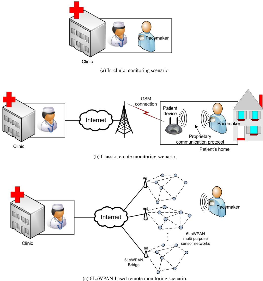
Fig. 1. Evolution of the implanted sensors monitoring scenario.
