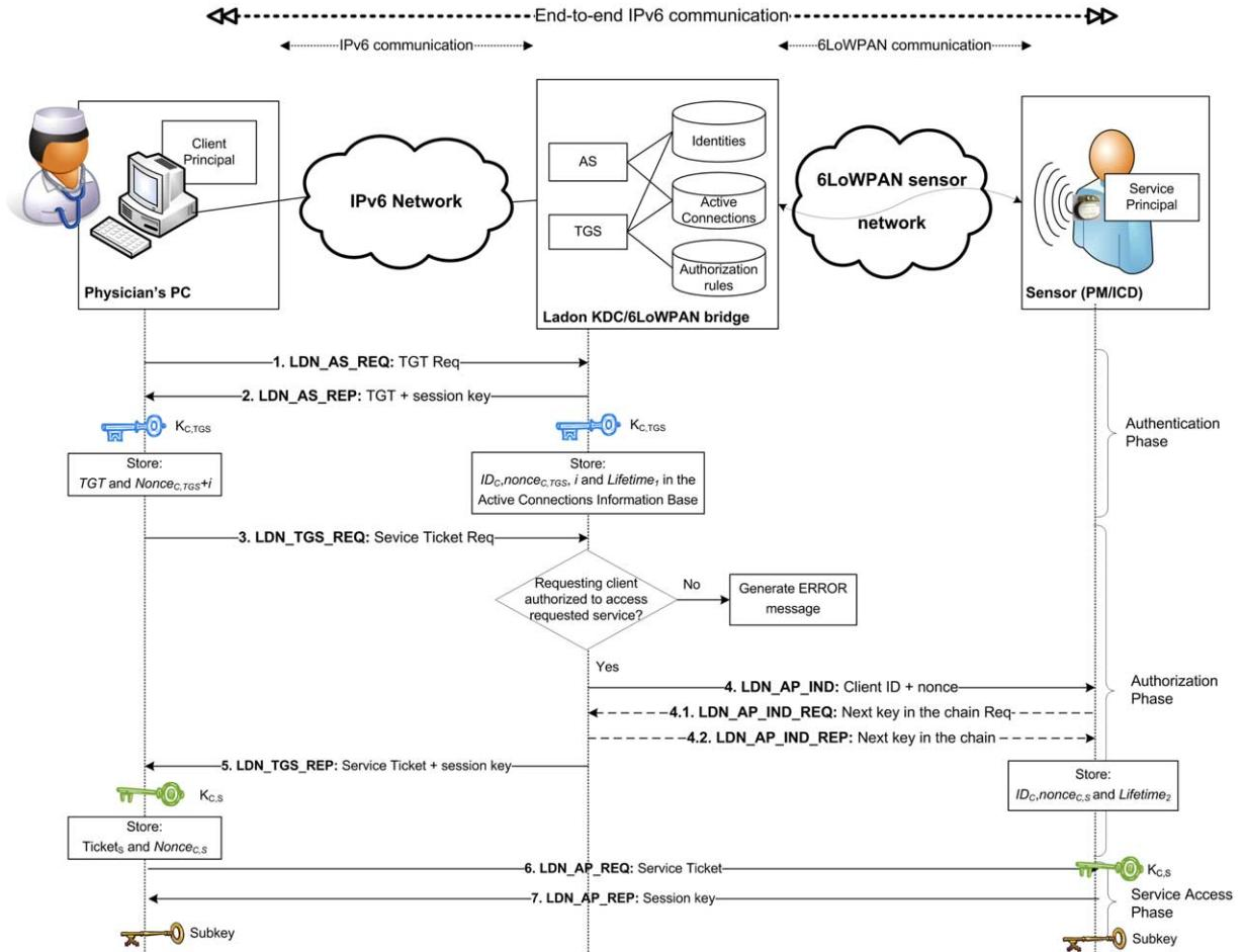
Fig. 3. Detailed operation and messages exchanged by the Ladon protocol.
