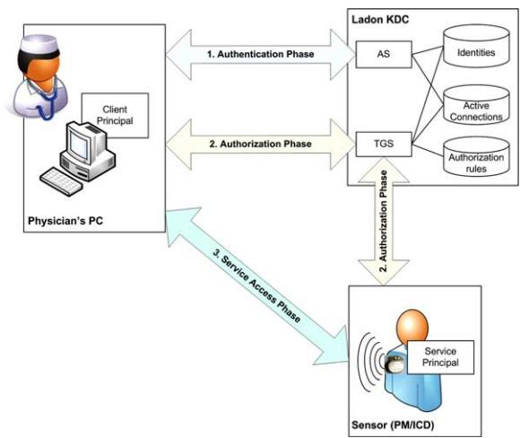
Fig. 2. Basic architecture and operation of the Ladon protocol.
