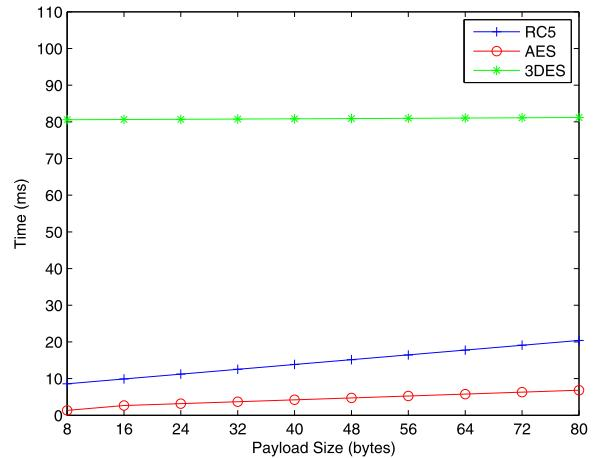
Fig. 5. Comparison of the time needed to encrypt different size payloads with 3DES, RC5 and AES block ciphers.
