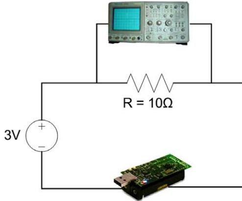
(a) Set-up for the measurement of energy consumption during data transmission
