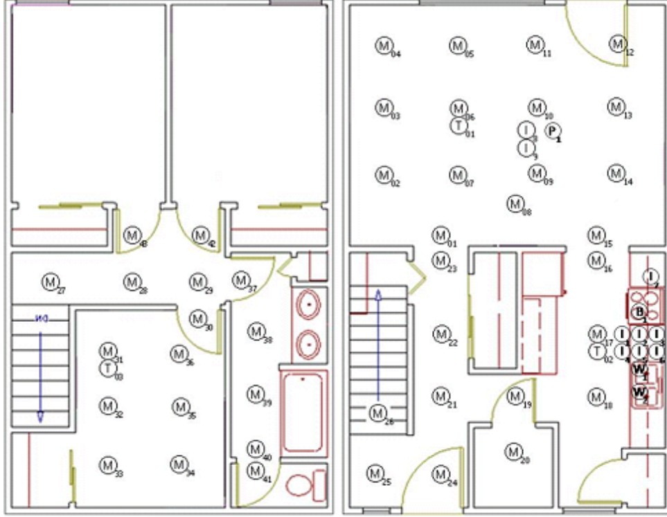
Fig. 4. Sensors in the WSU apartment test bed, monitor motion (M), temperature (T), water (W), burner (B), phone (P), and item use (I).
