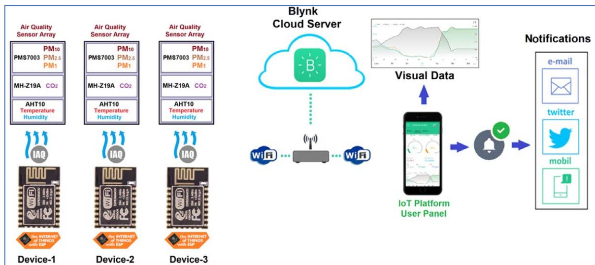
Fig. 3. The architecture of the IoT-based IAQ monitoring system for smart homes.
