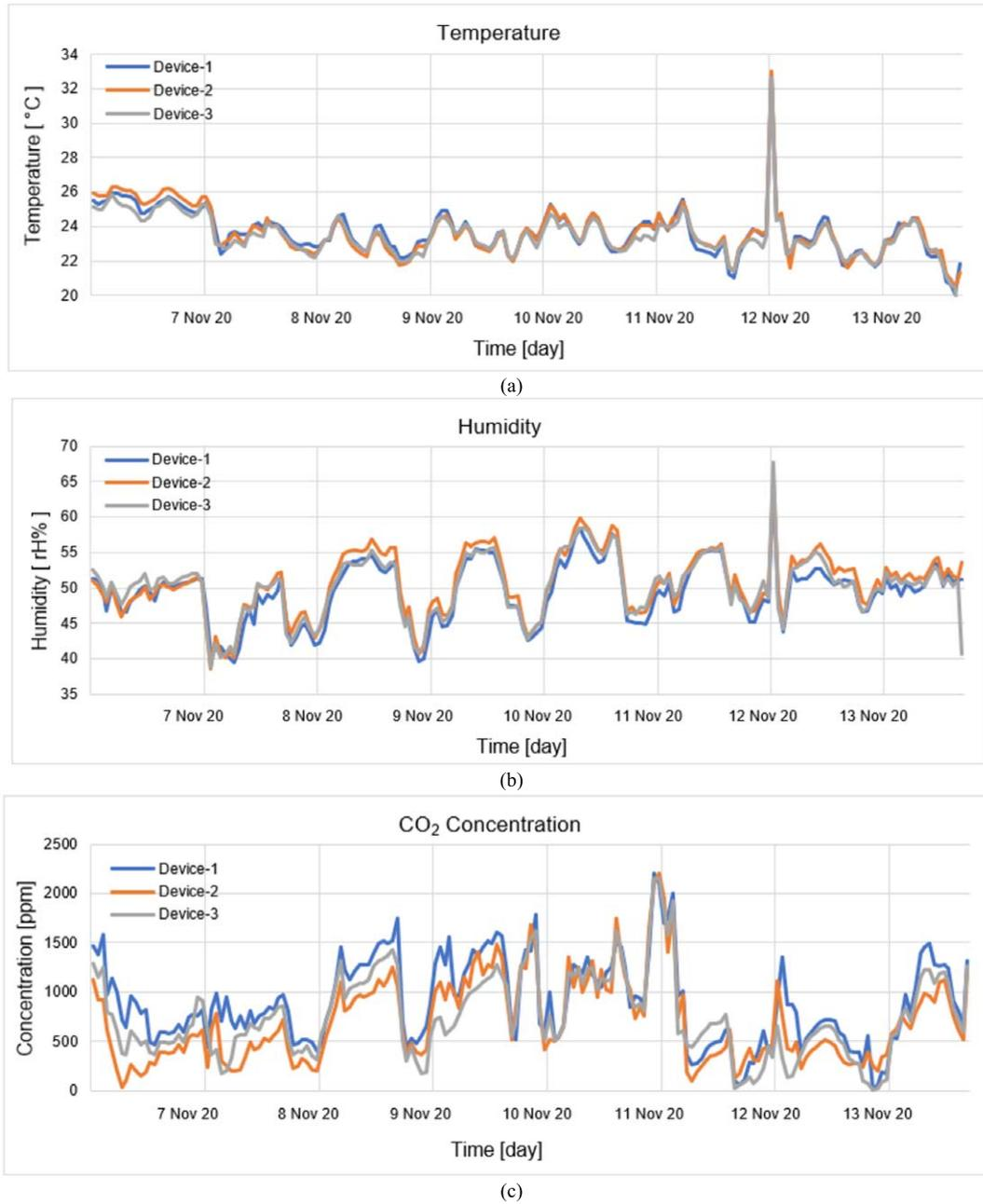
Fig. 9. Air quality parameters taken from the devices (a) temperature; (b) humidity; (c) CO<sub>2</sub> concentration.
