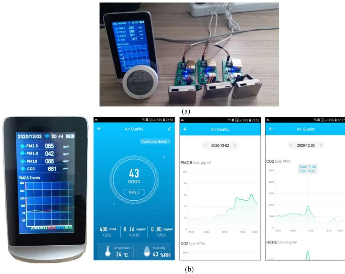
Fig. 7. (a) Calibration of air quality measuring devices with reference devices, (b) Screenshots of the Dienmern DM72B air quality monitor and Tuya Smart.
