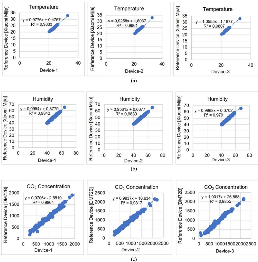
Fig. 10. SLR graphs of the devices; (a) temperature; (b) humidity; (c) CO<sub>2</sub> concentration.
