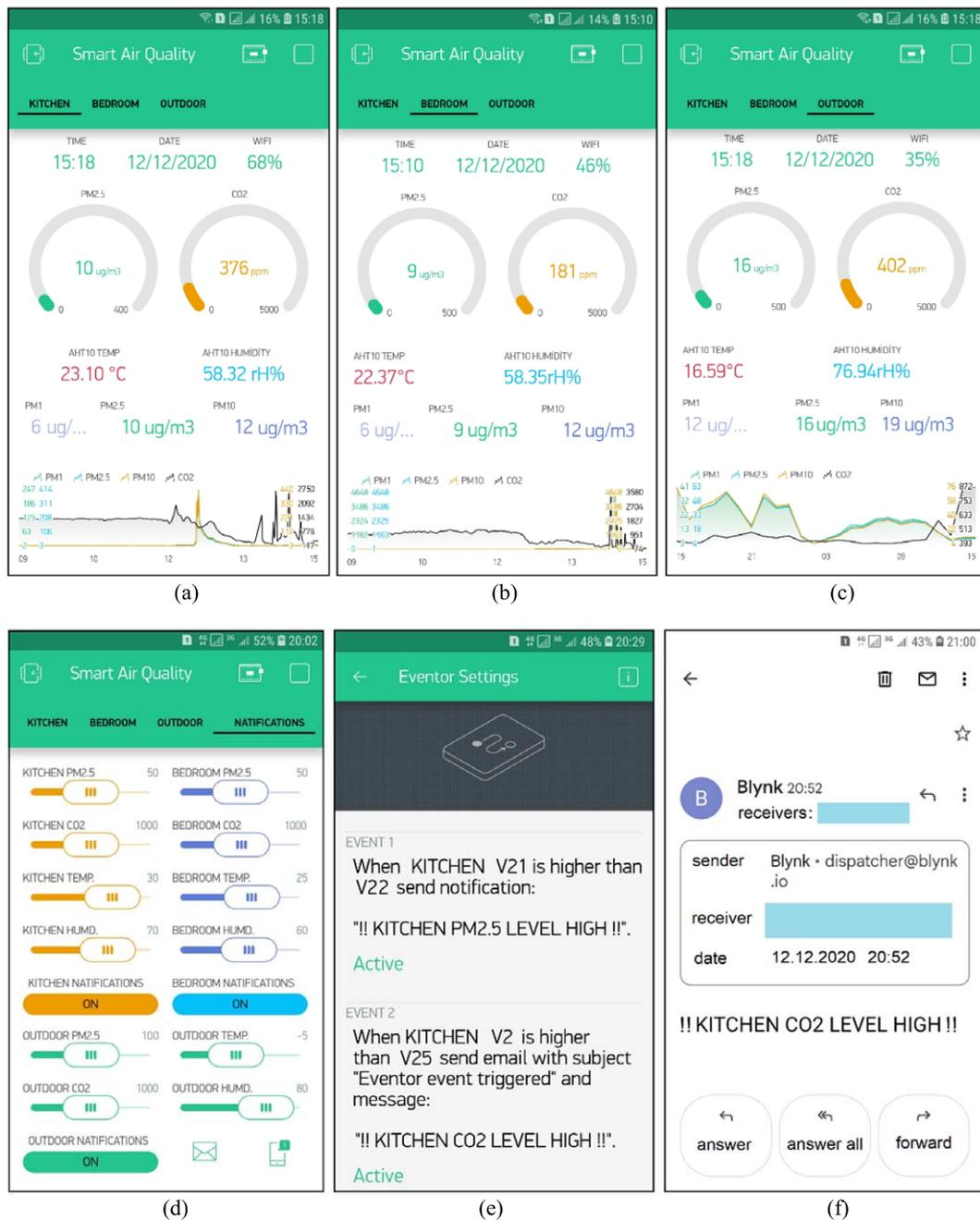
Fig. 5. The user interface of the air quality measurement device (a) kitchen, (b) bedroom, (c) outdoor, (d) notification setup, (e) eventor setup, (f) mail notification.
