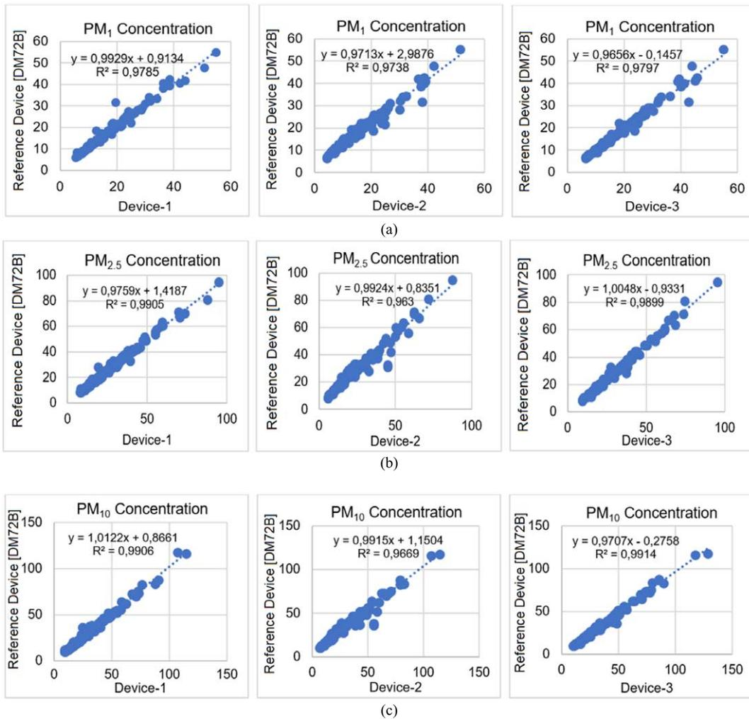
Fig. 11. SLR graphics of the devices, (a)  $PM_1$ , (b)  $PM_{2.5}$ , (c)  $PM_{10}$ .
