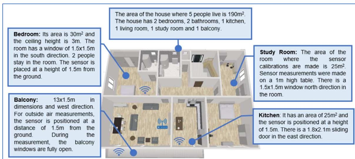
Fig. 2. House plan and sensor locations.
