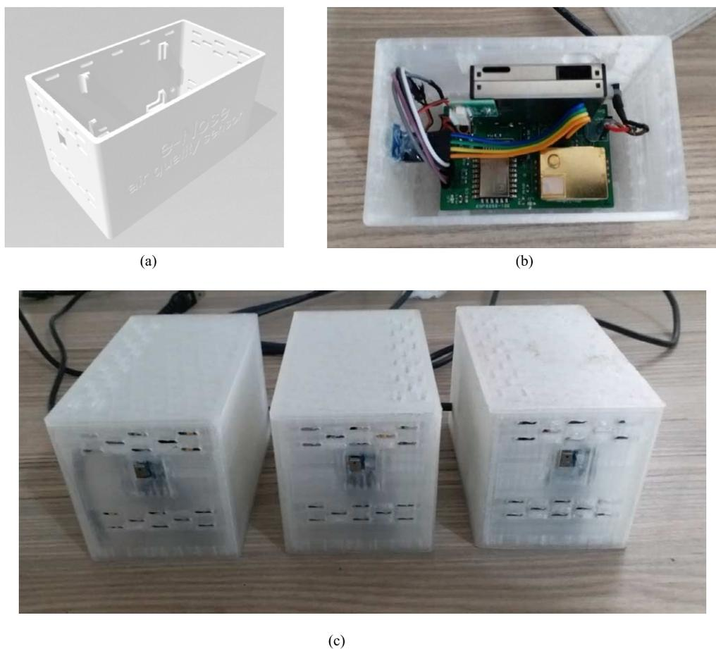
Fig. 4. Air quality measurement device (a) 3D box model, (b) in-box sensor assembly, (c) full assembled state.
