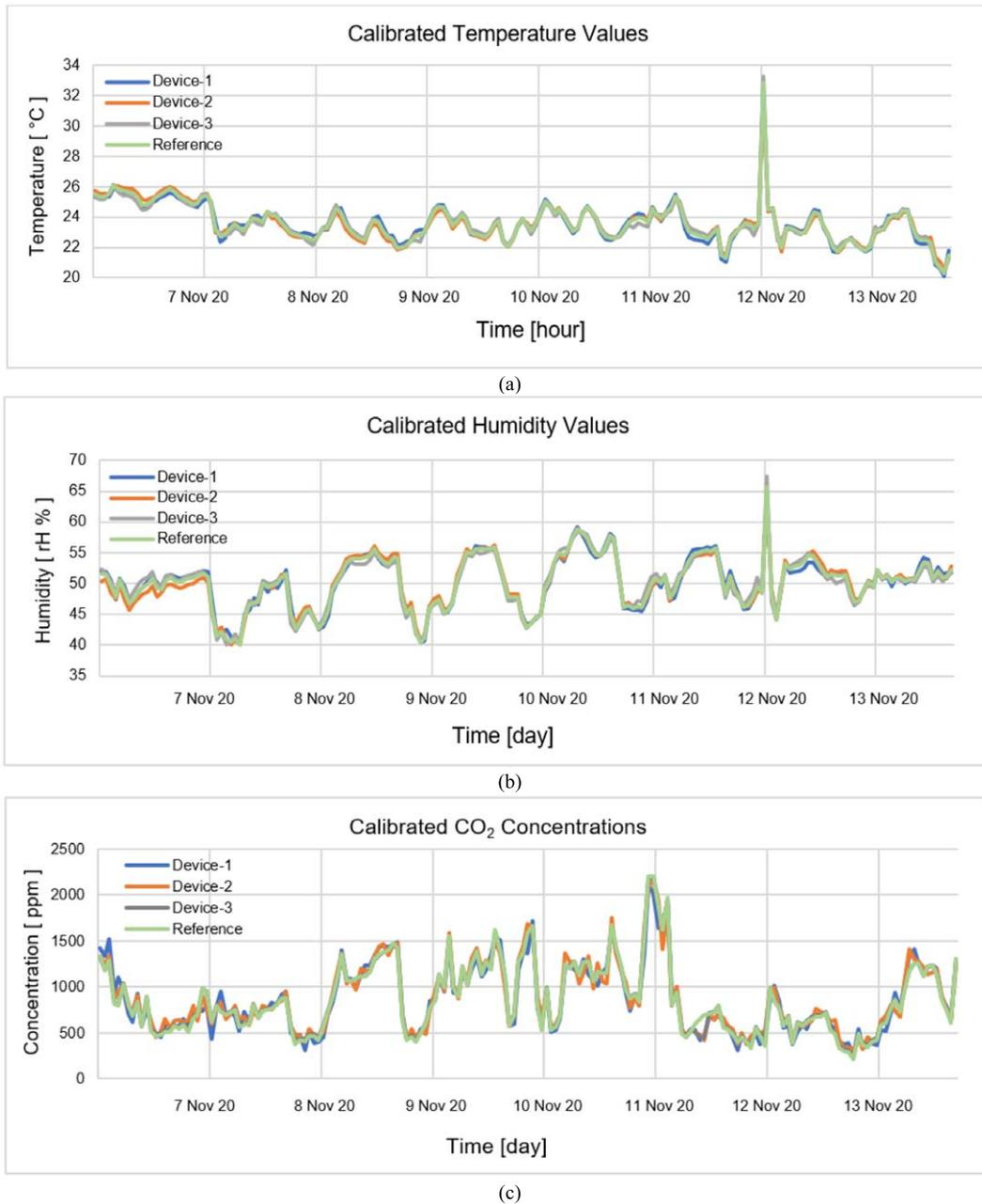
Fig. 13. Calibrated air quality parameters of the devices (a) temperature; (b) humidity; (c) CO<sub>2</sub> concentration.
