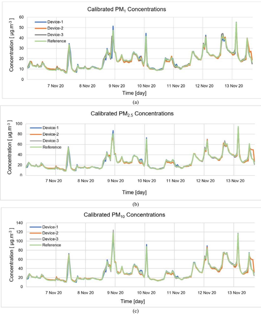
Fig. 12. Calibrated PM concentrations of devices (a) PM<sub>1</sub>, (b) PM<sub>2.5</sub>, (c) PM<sub>10</sub>.
