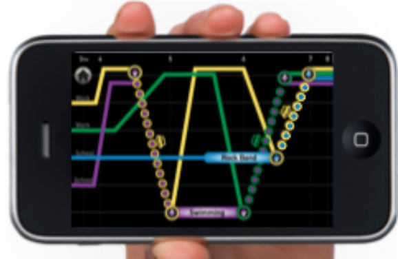
Fig. 2. The PPTV showing a simple plan. Rows are places, colored lines people. Lines are horizontal when a person is at a place, diagonal when traveling. Arrows indicate pick-ups and drop-offs, and dotted lines indicate parent-child co-travel.
