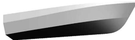
Fig. 16. Parent hull form DSDS  $25^\circ$ .
