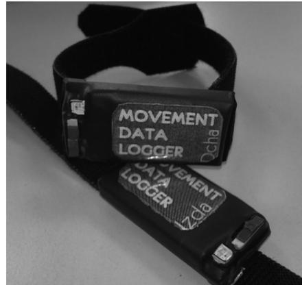
Fig. 4. The tri-axial bracelets used in this study, one for each hand.
