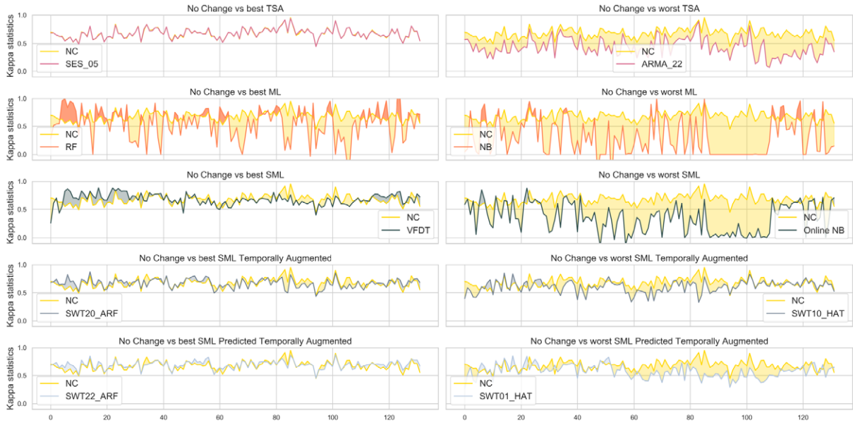
Fig. 3. Kappa statistics results achieved over all the segments. The first column compares the best TSA, ML, SML, SML Temporarily Augmented, and SML Predicted Temporarily Augmented models w.r.t. the Baseline (No Change classifier), while the second column compares the worst TSA, ML, SML, SML Temporarily Augmented, and SML Predicted Temporarily Augmented models w.r.t. the Baseline.
