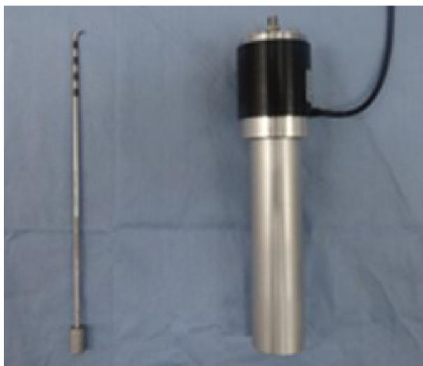
Fig. 2. Shows two components of the probing device in the current study. Left one is the probe with a half size. Four black marked parts in the tip of the probe are to measure a distance of tissues on the monitor. The distance of each part is 5 mm. Right one is main component to measure the force. 3-axis load cell is embedded in the black measurement part. The grip part is connected with the measurement part.
