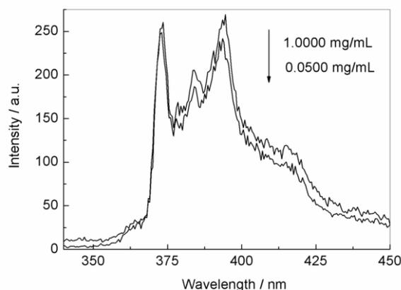
Fig. 4. Fluorescence emission spectra of pyrene as a function of PHCSO-g-PCL concentration.
