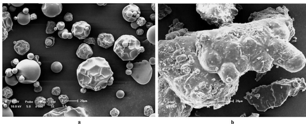
Fig. 3. SEM analysis of (a) CSO and (b) PHCSO-g-PCL ( $\times 500$ ).
