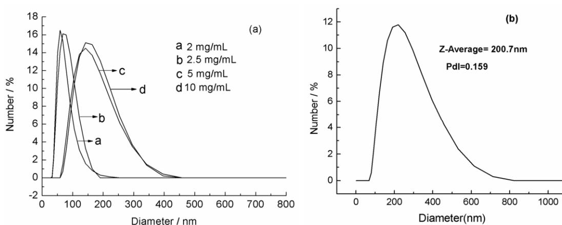
Fig. 5. Size and size distribution of PHCSO-g-PCL particles with (a) various concentrations and (b) BSA drug.
