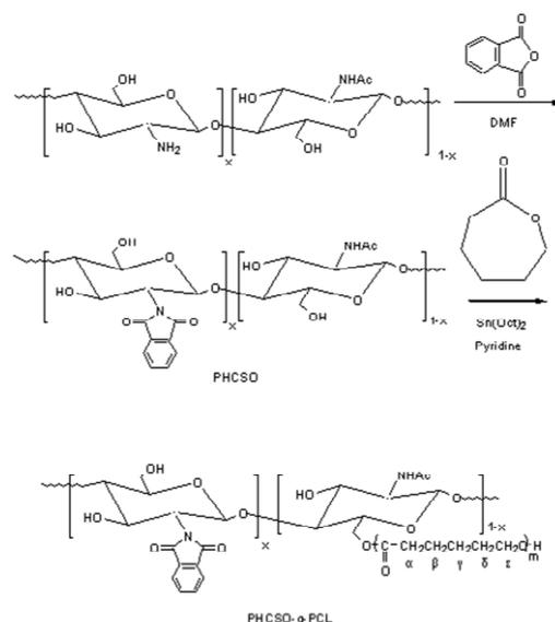
Fig. 1. Synthetic procedure of PHCSO-g-PCL.
