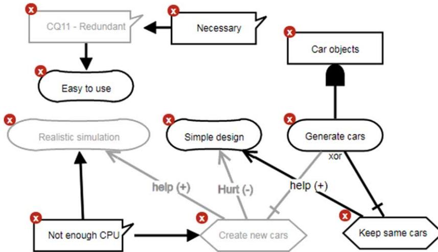
Fig. 22. Adding an argument that attacks multiple GRL elements to Fig. 20.
