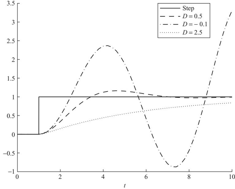
Fig. 2. Response of a  $PT_2$  system to a step function with exemplary values for  $D$
