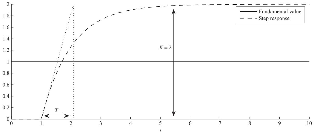
Fig. 1. Response of a  $PT_1$  system to a step function
