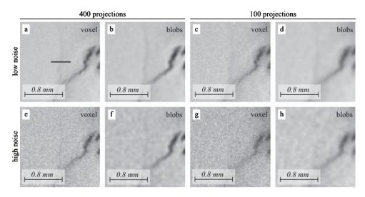
Fig. 6. Comparison of a small crack. a) lownoise400 voxel based, additionally, the line for the line profile is depicted, b) lownoise400 blob based, c) lownoise100 voxel based, d) lownoise100 blob based, e) highnoise400 voxel based, f) highnoise400 blob based, g) highnoise100 voxel based, and h) highnoise100 blob based.
