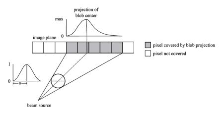
Fig. 3. Geometry of the back projection operation. The parallel projection of a three dimensional blob onto a two dimensional grid is a blob with the same radius as the original blob. However, a perspective projection can cover an area on the image plane much larger than the blob itself and is not symmetric in general.
