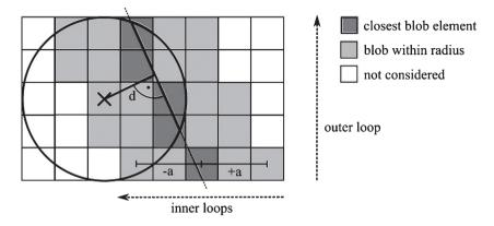
Fig. 2. Forward projection algorithm including slice stepping using blobs. For each pixel in the projection image the line integral of a line through this pixel is computed using nested loops. The outer loop iterates slices in the primary line direction. For each slice, the blob closest to the line is determined and all blobs within radius a are iterated. For each blob, the line integral is determined by means of a lookup dependent on the distance d between blob center and line.
