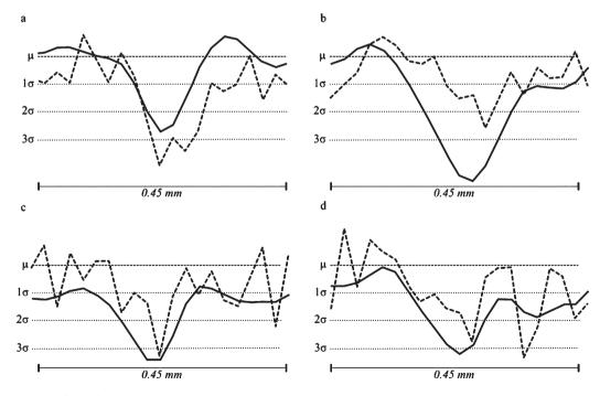
Fig. 7. Line profiles of the small crack. Dashed line: voxel based reconstruction and solid line: voxelized blob based reconstruction. Additionally, dotted lines for mean ( $\mu$ ) and standard deviations ( $\sigma$ ) of one, two, and three are shown. a) lownoise400, b) lownoise100, c) highnoise400, and d) highnoise100. Due to normalization, x- and y-axis have the same spacing ( $\mu = 0$ ,  $\sigma = 1$ ).
