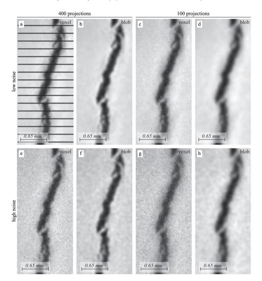
Fig. 5. Comparison of a big crack. a) lownoise400 voxel based, additionally, line profiles for the line analysis are depicted, b) lownoise400 blob based, c) lownoise100 voxel based, d) lownoise100 blob based, e) highnoise400 voxel based, f) highnoise400 blob based, g) highnoise100 voxel based, and h) highnoise100 blob based.
