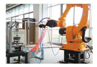
Fig. 1. The deburring industrial robot system.
