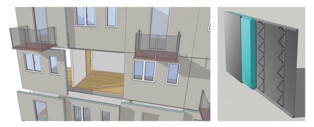
Fig. 1. SESBE facade concept (left) and innovative sandwich facade element (right).
