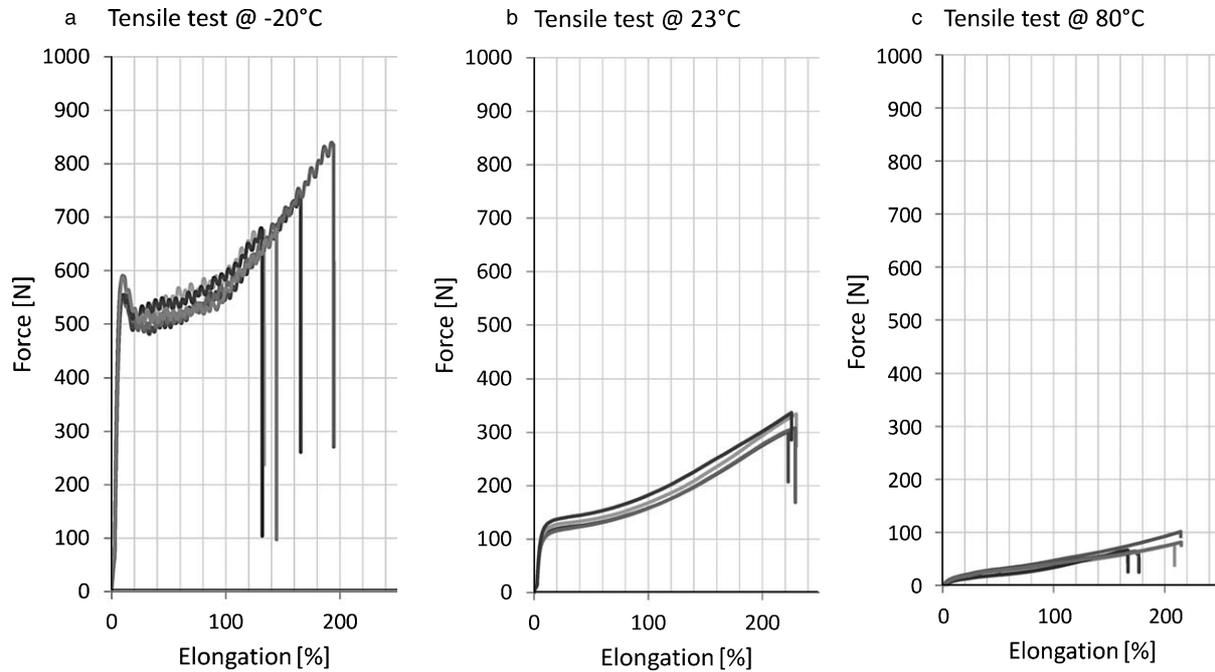
Fig. 6. Tensile test of mono-component acrylic at (a)  $-20^{\circ}\text{C}$ , (b)  $+23^{\circ}\text{C}$  and (c)  $+80^{\circ}\text{C}$ .
