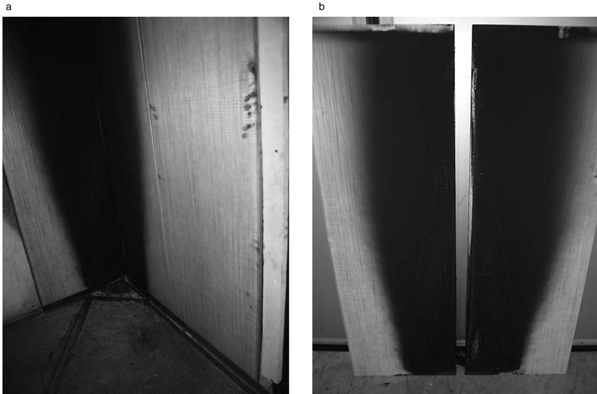
**Fig. 12.** SBI corner test performed with the final facade configuration. As can be seen, with materials of limited combustibility (class B) there is very limited fire spread in vertical direction and none in horizontal direction.
