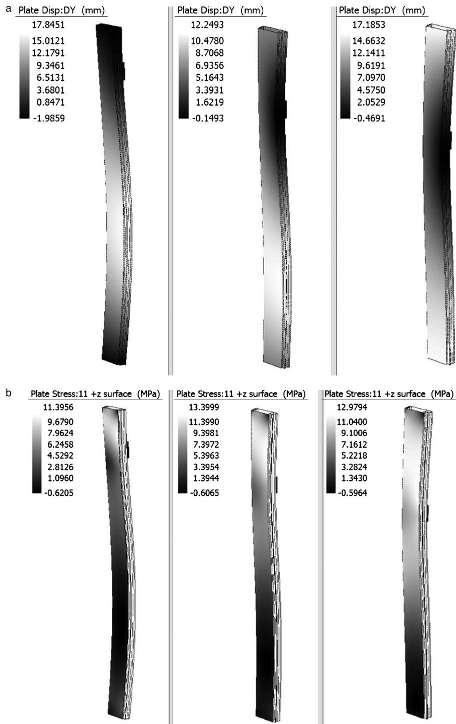
**Fig. 5.** FE results – influence of bracket position (from left, 500 mm, 850 mm and 1200 mm below the stack joint) on (a) deformation shape (b) distribution of principal tensile stress in glass.
