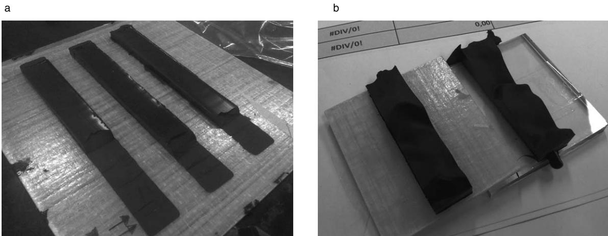
Fig. 8. Failure mode (a) peeling test (b) tensile test.
