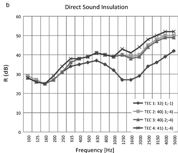
Fig. 9. Acoustic test (a) specimen set-up (b) direct sound insulation test results.
