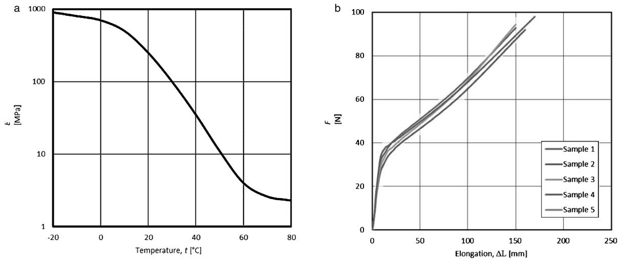
Fig. 7. Test results of bi-component acrylic adhesive (a) DMA test (b) tensile test at 23°C.
