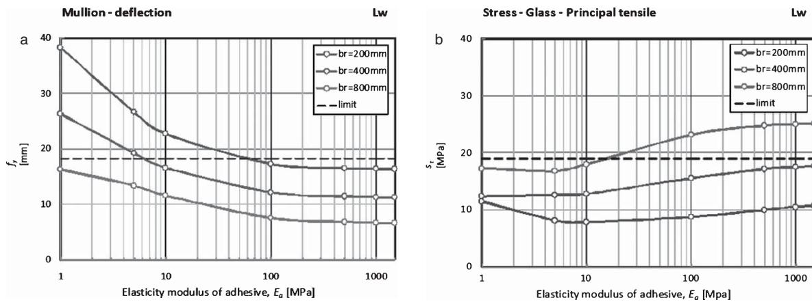
**Fig. 4.** FE results – influence of elasticity modulus of adhesive  $E_a$  on (a) out-of-plane mullion deflection  $f_y$ , (b) principal tensile stress in glass  $\sigma_t$ .
