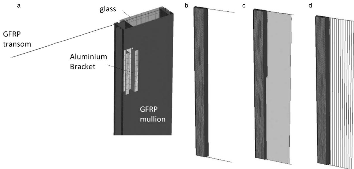
**Fig. 3.** FE modelling: (a) connection details (b) symmetrical model (c) load path (d) Gerber effect.
