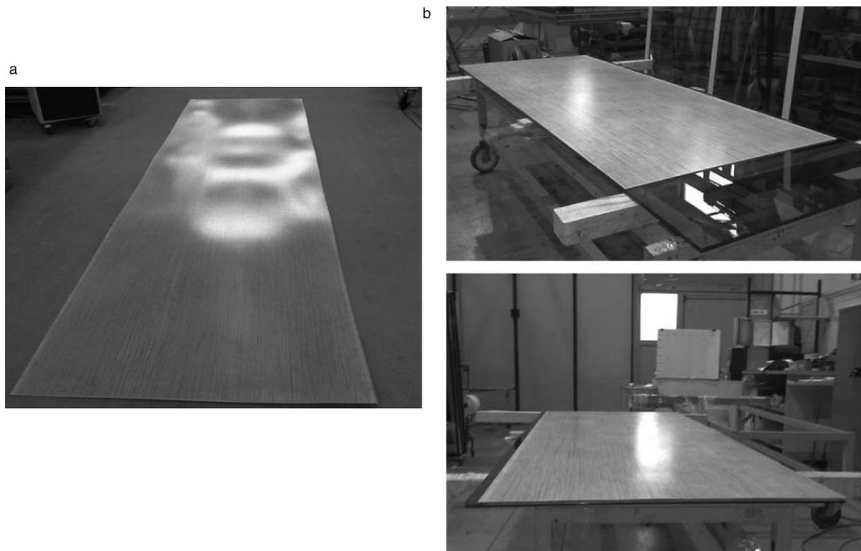
**Fig. 11.** 3 mm GFRP plate flatteners (a) before lamination (b) after lamination.
