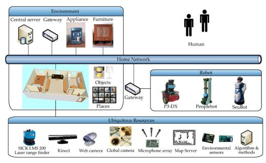
Fig. 8. The experimental system for ambient assisted living application.
