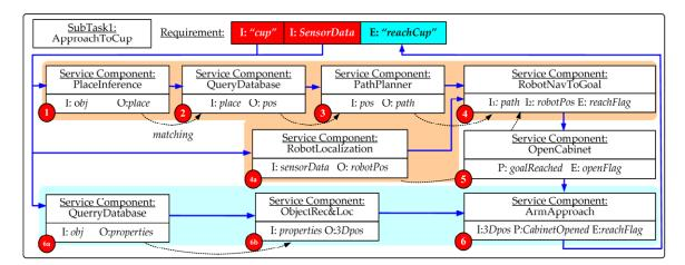
Fig. 9. Example of assembling services SubTask1 of the "CupFetching" scenario.
