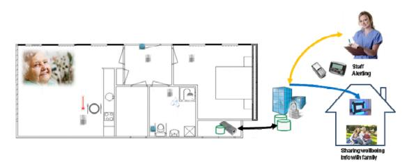
Fig. 5. Third generation of the Aurama awareness system: towards less obtrusive sensing and involving formal care providers.
