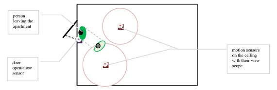
Fig. 6. Detecting home presence using distributed multimodal sensors.
