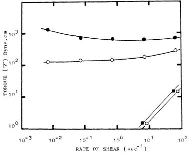
Fig. 17. Comparisons of torque values from surface layers of  $-\bullet - 0.4\%$  bovine fibrinogen and  $-\Box - 0.25\%$   $\beta$ -lipoprotein as controls. -0-0.4% fibrinogen plus 0.025%  $\beta$ -lipoprotein;  $-\blacksquare - 0.4\%$  fibrinogen plus 0.25%  $\beta$ -lipoprotein.
