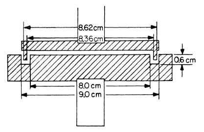
Fig. 7. Plan view of special geometry for direct measurements of rheological properties in steady or oscillatory shear of surface layers.
