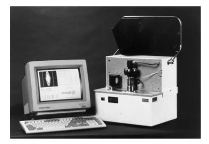
Fig. 2. Laser-assisted Optical Rotational Cell Analyser (LORCA).
