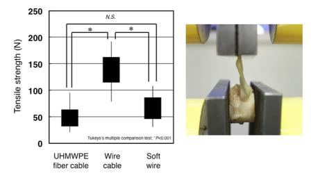
Fig. 2. The pull-out strength at the insertion site of various fixation materials. The right photograph shows how the test was carried out in the UHMWPE fiber cable sample. The ultimate failure load using a UHMWPE fiber cable, wire cable, or soft wire is shown in the left graph. The results are expressed as the mean  $\pm$  standard deviation. (Colors are visible in the online version of the article; http://dx.doi.org/10.3233/BME-130757.)
