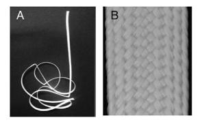
Fig. 1. Photograph of the UHMWPE fiber cable. (A) Gross appearance. (B) Close-up appearance (original magnification  $\times$ 30). The cable is a soft flexible material in the form of a tape.
