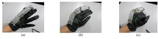
Fig. 5. CPM rehabilitation experiment of joints PIP and DIP of ring finger.
