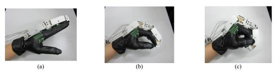
Fig. 4. CPM rehabilitation experiment of joints PIP and DIP of middle finger.
