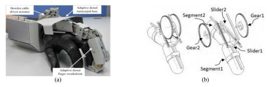
Fig. 1. Hand rehabilitation exoskeleton: (a) overall structure. (b) SPRM with the parallel mechanism.
