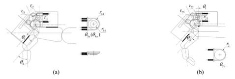
Fig. 3. Structure of joints: (a). One-DOF SPRM with parallel mechanism. (b). Two-DOF SPRM with parallel mechanism.
