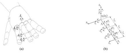
Fig. 2. The coordinate establishing method of the middle finger: (a) The DOF analysis of the middle finger. (b) The coordinates of the links of the middle finger.
