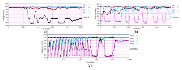
Fig. 8. The signals of the force sensors during typical motions: (a) The independent slow bending of joint MCP-2. (b) The coupling intermittent bending of joints PIP and DIP. (c) The intermittent natural bending of the finger.
